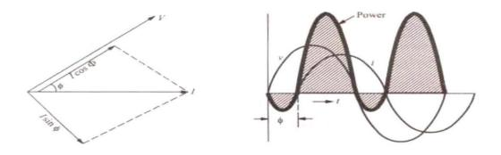
The mean power consumed by the circuit is given by the product of V and that component of the current I which is in phase with V So P = V X I cos  $\Phi$  = r.m.s. voltage X r.m.s. current X cos  $\Phi$ The term cos  $\Phi$  is called the power factor of the circuit
