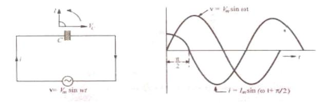
Now, current I is given by the rate of flow of charge.
