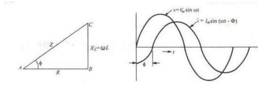
IIn fig. I has been resolved in to its two mutually perpendicular components, I cos  $\Phi$  along the applied voltage V and I sin  $\Phi$  in quadrature (i.e. perpendicular) with V.
