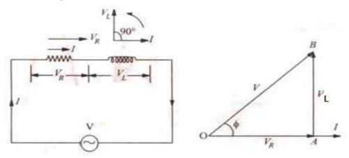
Let V = r.m.s. value of the applied Voltage, I = r.m.s. value of the resultant current  $V_R$  = IR – Voltage drop across R ( in phase with I),  $V_L$  = I.X<sub>L</sub> – voltage drop across coil (ahead of I by 90<sup>0</sup>)
