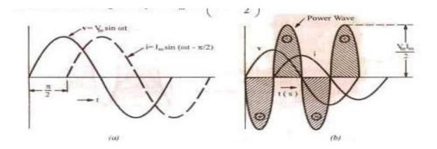
Clearly, the current lags behind the applied voltage by a quarter cycle (fig) or the phase deference between the two is  $\frac{\pi}{2}$  with voltage leading. Vectors are shown in fig. where voltage has been taken along the reference axis. We have seen that
