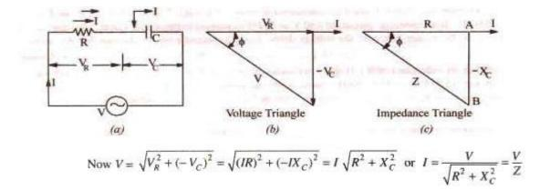
The denominator is called the impedance of the circuit. So  $Z = \sqrt{R^2 + X_c^2}$ Impedance triangle is shown in fig.
