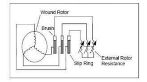
This type of rotor is provided with  $3-\phi$ , double-layer, distributed winding consisting of coils. The rotor is wound for as many poles as the number of stator poles and is always wound 3phase even when the stator is wound two-phase. The three-phases are starred internally and the construction is complicated.
