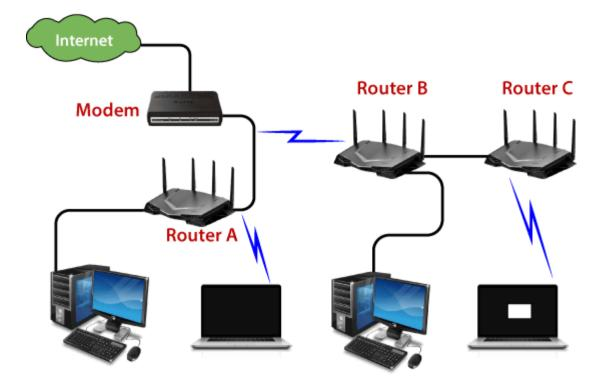
**Modem** is short for "**Modulator-Demodulator**." It is a hardware component that allows a computer or another device, such as a router or switch, to connect to the Internet. It converts or "modulates" an analog signal from a telephone or cable wire to digital data (1s and 0s) that a computer can recognize.
