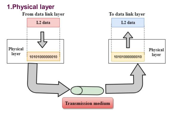
• The main functionality of the physical layer is to transmit the individual bits from one node to another node.
