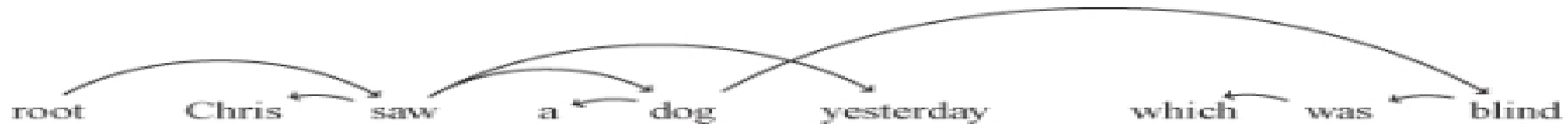
Figure 3–3. An unlabeled nonprojective dependency tree with a crossing dependency
